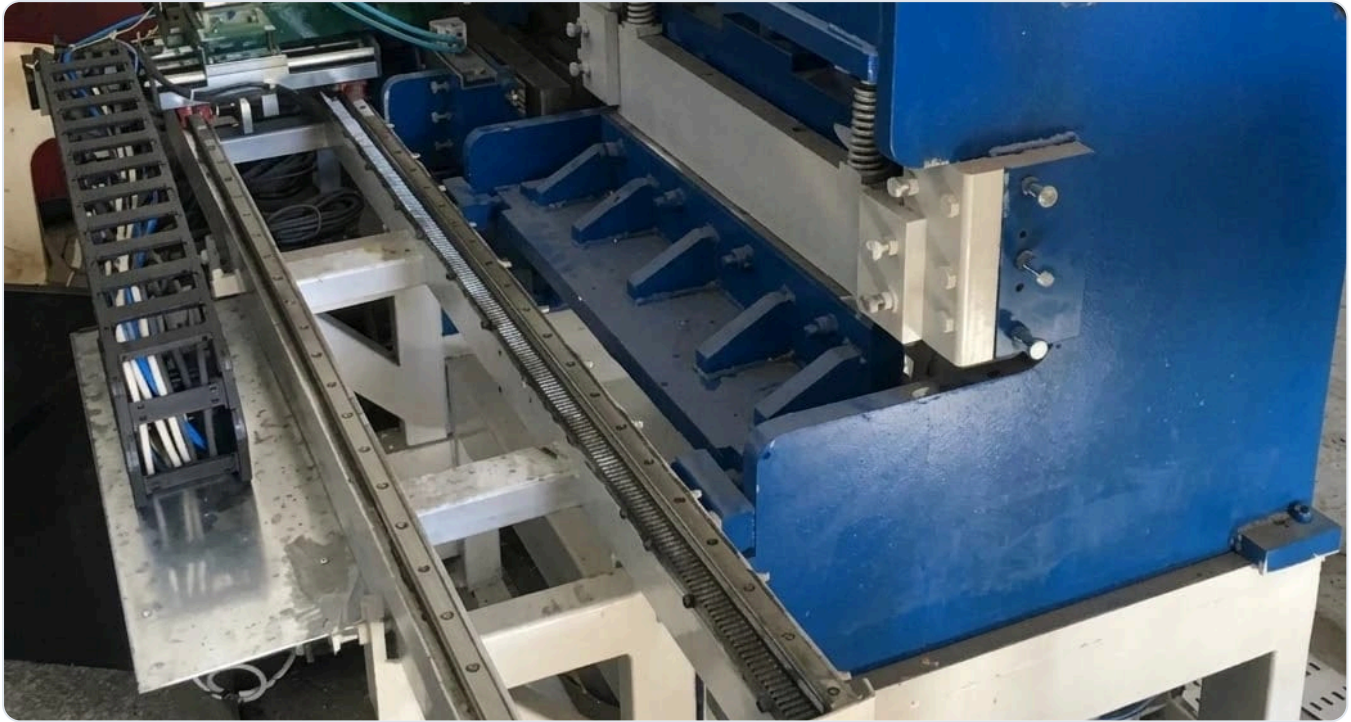
Transfer press in the workshop — 2-axis linear robot rail, cable chain and hydraulic press frame, real photo
