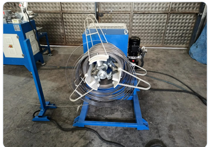
Uncoiler with hydraulic motor, loaded with a wire coil
