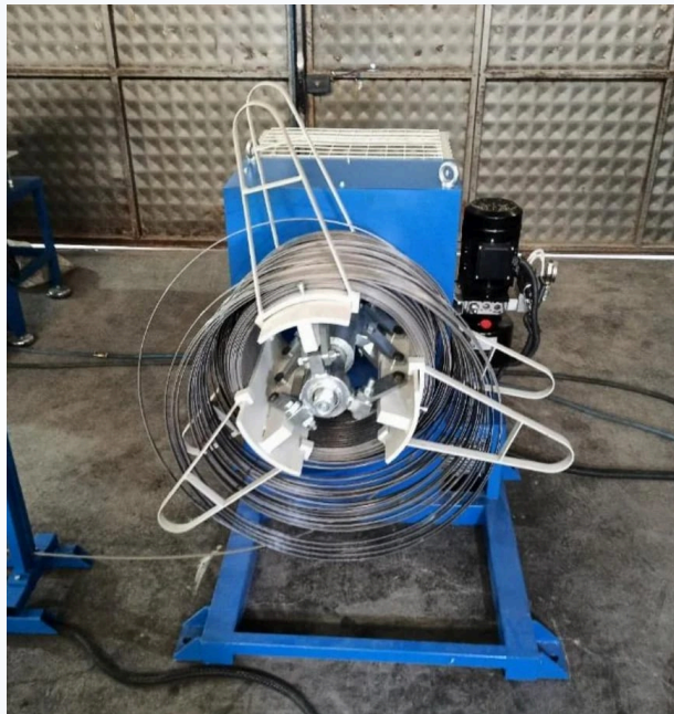
Uncoiler with hydraulic mandrel and control panel
