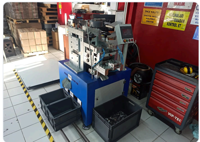
Rotary Punch chopping and marking machine installed at a production plant, with HMI panel and product crates
