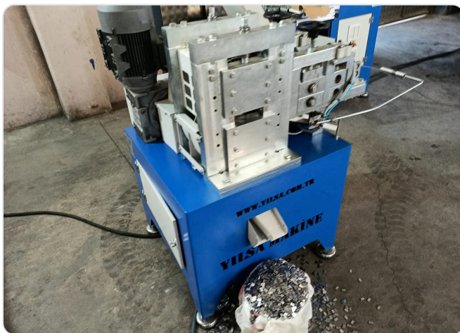
YILSA-branded Rotary Punch chopping and marking machine — motor and twin-drum die block
