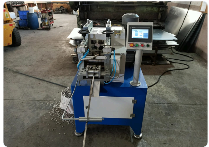
Rotary Punch chopping and marking machine running in the workshop, with cut wheel weights in a bucket
