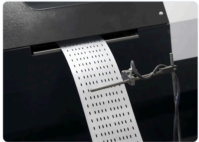
Close-up of sheet with oval holes punched by Rotary Punch leaving the machine
