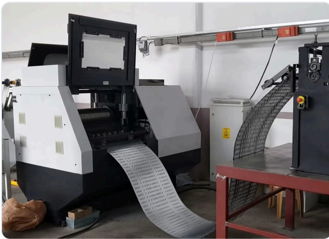
Rotary Punch punching unit running in the workshop, with perforated sheet coming out and the straightening unit — real photo
