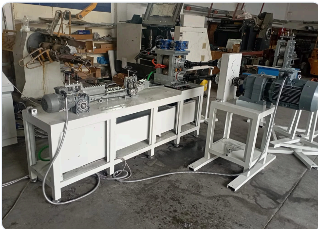
Wire rod flattening machine in the workshop — wire straightening inlet, flattening rolls and drive motor, real photo
