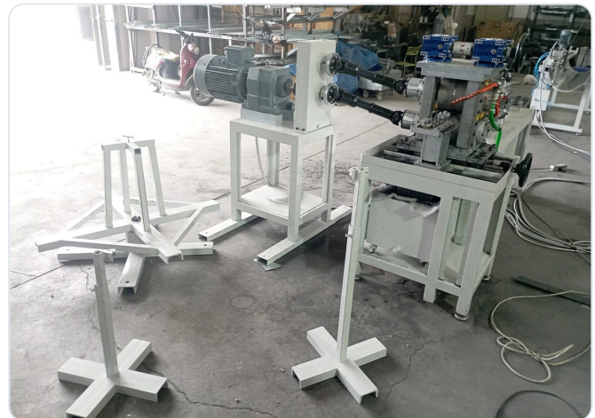
Wire rod flattening machine — flattening unit, geared drive and wire guide stands
