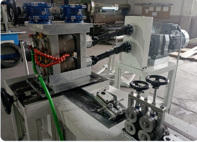
Close-up of the wire flattening rolls, central clamping handwheels and coolant hose
