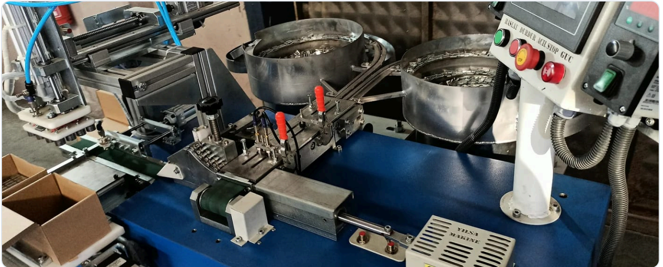
Vibratory feeders, taping line and control panel
