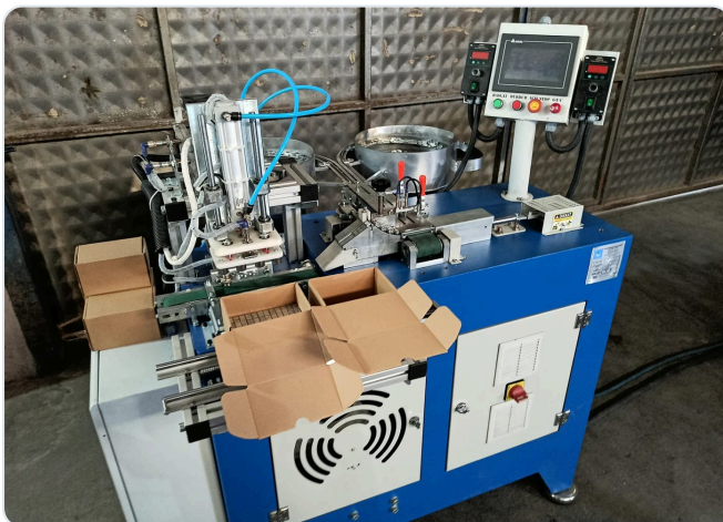
Taping and packaging machine with vibratory feeders and box filling station
