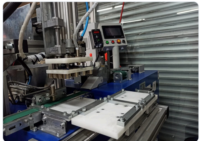
Close-up of the pneumatic placing head and packaging table of the taping and packaging machine
