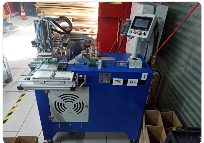
Taping and packaging machine installed at a production plant, with HMI panel
