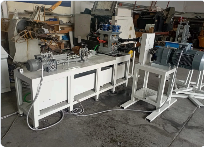
Wire rod flattening machine in the workshop — wire straightening inlet, flattening rolls and drive motor, real photo
