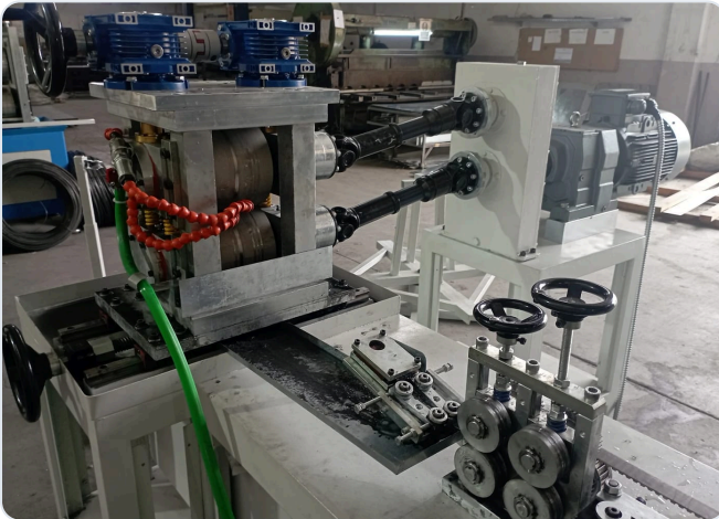
Close-up of the wire flattening rolls, central clamping handwheels and coolant hose
